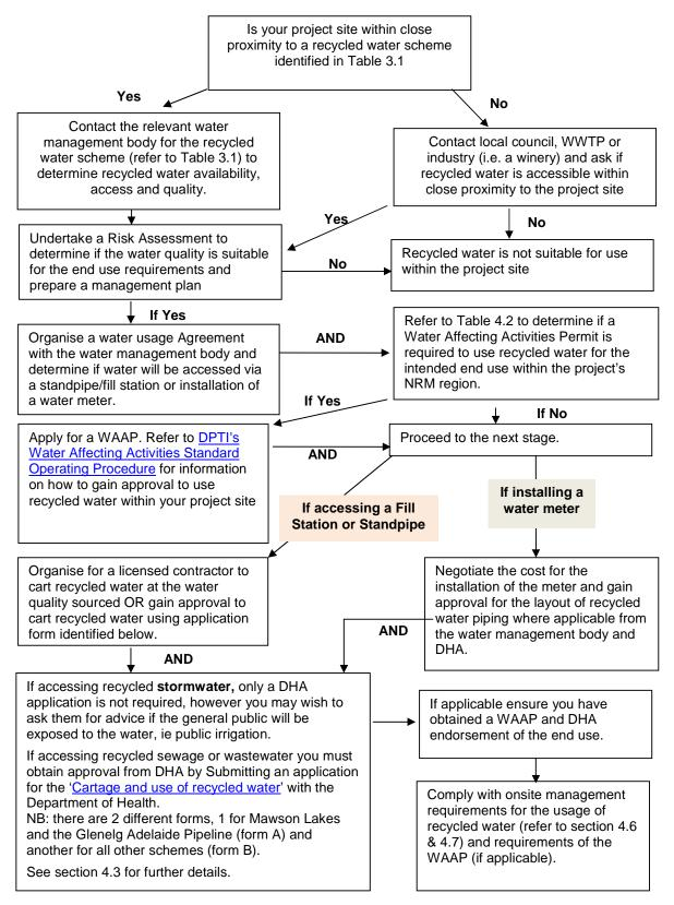
Figure 4.1: Procedure for the use of recycled water
